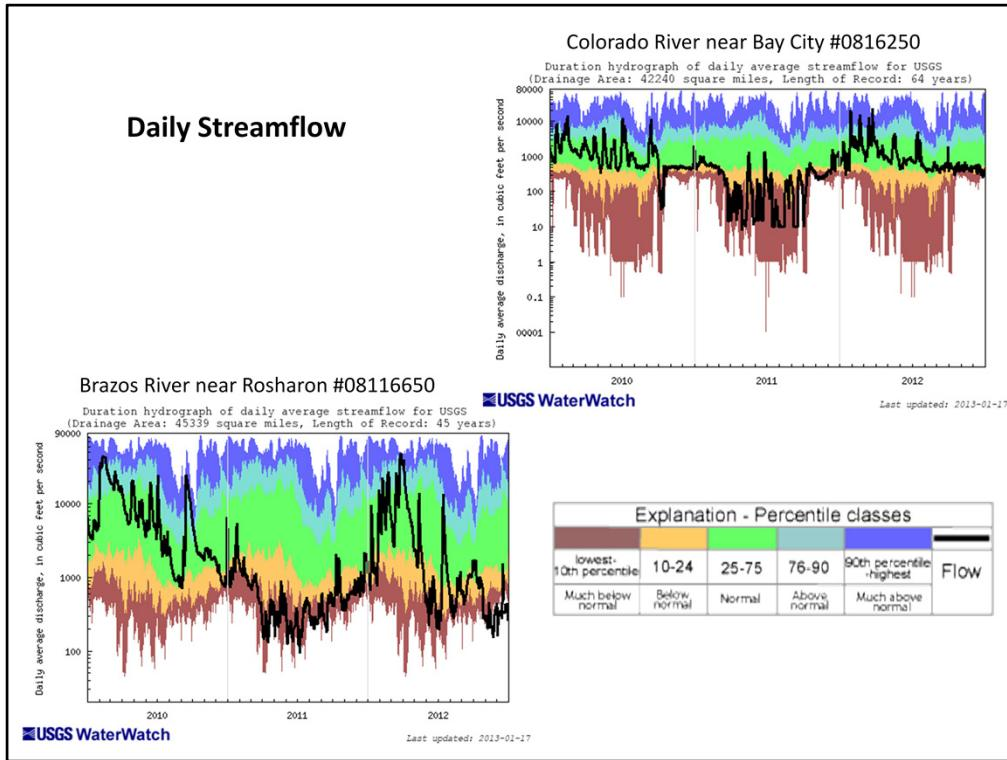
This slide shows two examples of streamflow volumes during 2011 as compared to flows during other years. Admittedly, I selected the most astounding gages to showcase here.... You can see on the Colorado River near Bay City (TOP RIGHT), streamflows plummeted during the end of 2010 through 2011, typically falling within the lowest 10<sup>th</sup> percentile (MUCH below normal).
