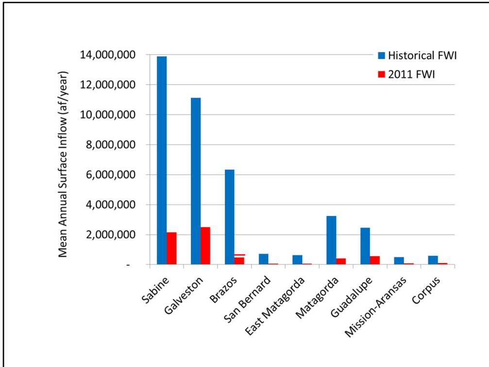
\*Preliminary data\* \*Does not include diversion and return flow data for any basin; Brazos is “gage only” but red line estimates gage + modeled using avg modeled inflow over the period of record\* \*Laguna Madre inflows are still being developed\*
